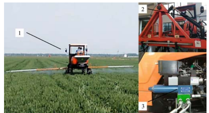
1. Self-propelled sprayer 2. Active pendulum boom suspension 3. Electro-hydraulic servo control valve
